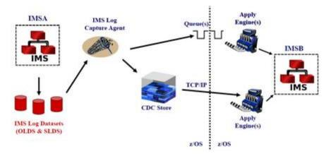
Figure 6: Log-based capture
