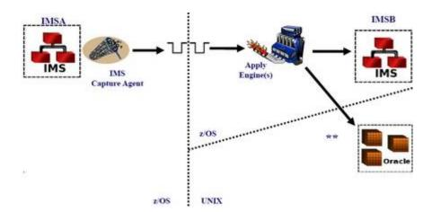
Figure 3: Active/Passive replication
