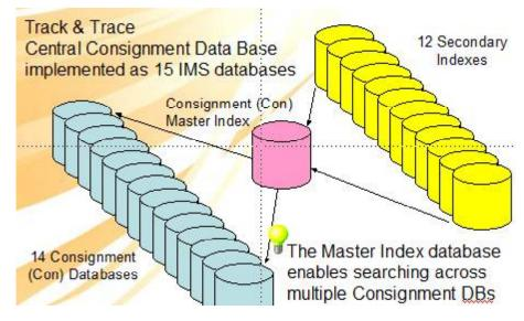
Figure 2: Application partitioning - CCDB
