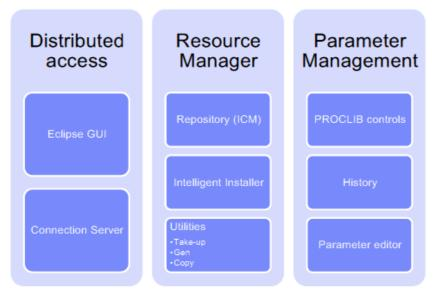
Figure 1: Components of IMS Configuration Manager
