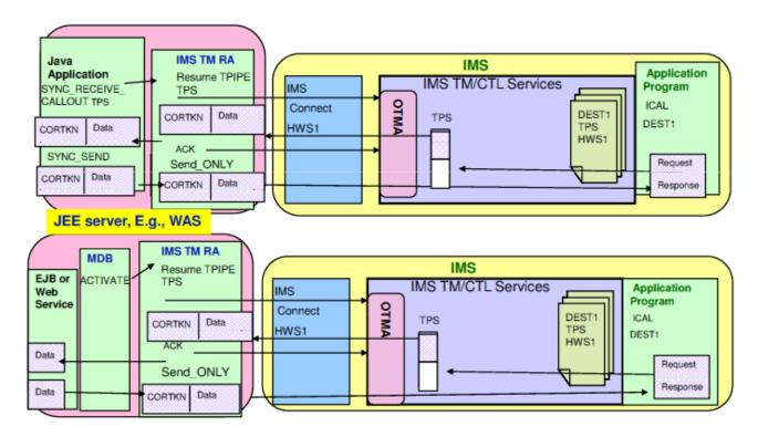
Figure 2: IMS TM Resource Adapter (JEE environments)
