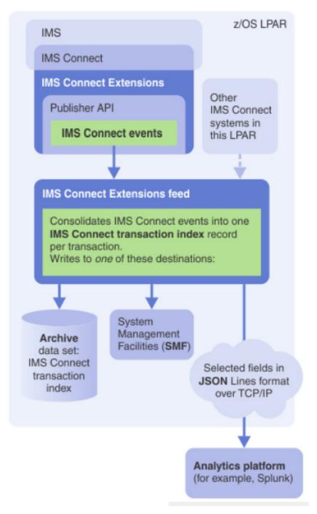
Figure 4: IMS Connect Extensions feed
