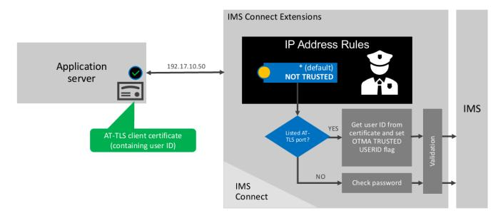
Figure 3: Security: take the user ID from the client's digital certificate (AT-TLS)
