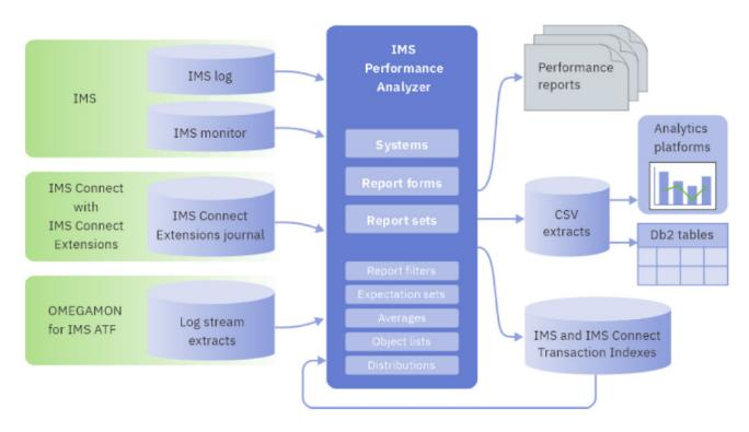
Figure 3: IMS Performance Analyzer V4.5
